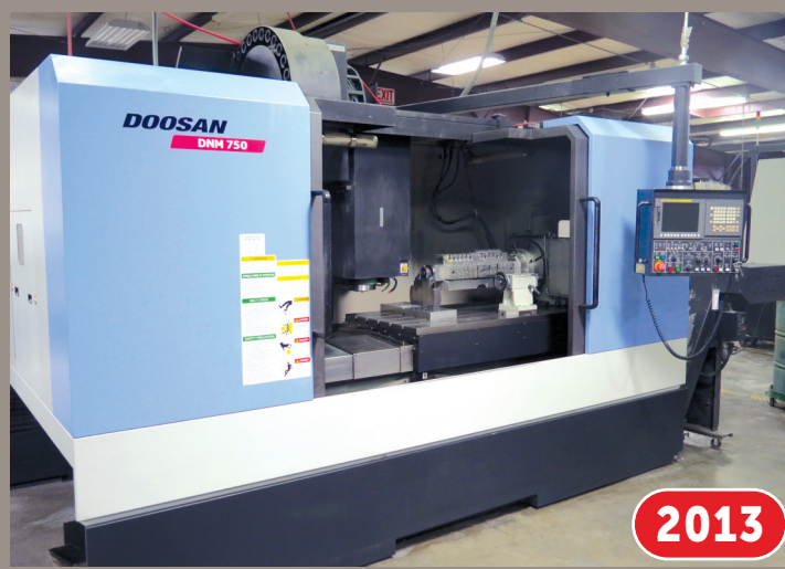
Doosan DNM750 4-Axis VMC, Fanuc 30i Control
