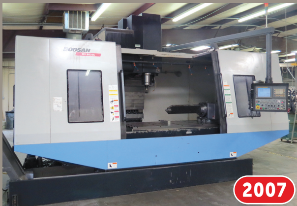
Doosan MV8035S 4-Axis VMC, Fanuc 18i-MB Control
