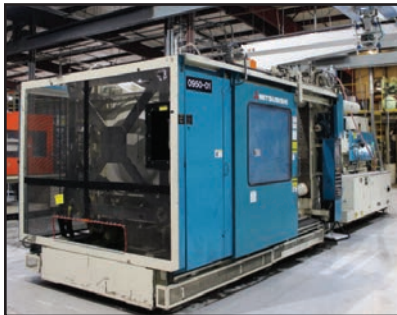
950-Ton Mitsubishi 950MMJW-160 Injection Molder
