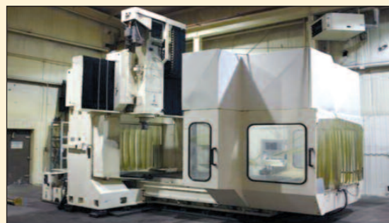
Nicholas Correa FP40/30 CNC Bridge Mill
