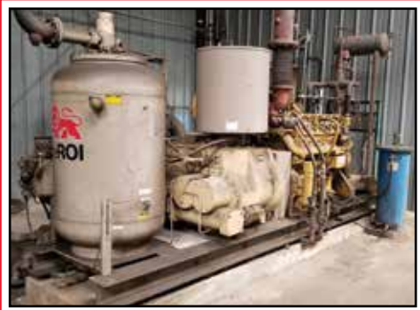
(4) LEROI 600-HP Gas Powered Rotary Screw Air Compressors w/CAT 3412 NG 600+ HP Engines
