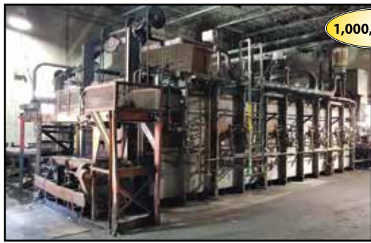
Heat Treat Line - (2) ELECTRIC FURNACE CO. 52'W x 30'L x 12"H Natural Gas Fired Pusher Furnaces
