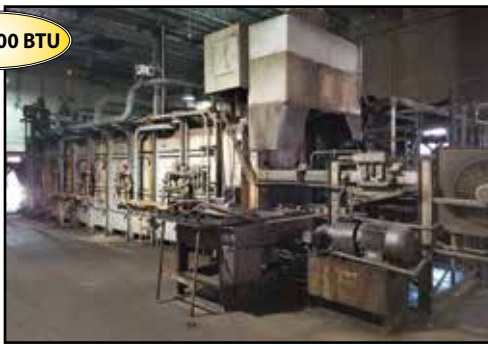
Heat Treat Line - (2) ELECTRIC FURNACE CO. 52'W x 30'L x 12"H Natural Gas Fired Pusher Furnaces
