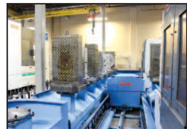
(2) Mazak PFH-5800, 4-Axis Pallettech F.M.S., Fusion 640M Controls, (10) 20" Pallets, 15k RPM, 80 ATC, CTS, Probe, Chip Blaster
