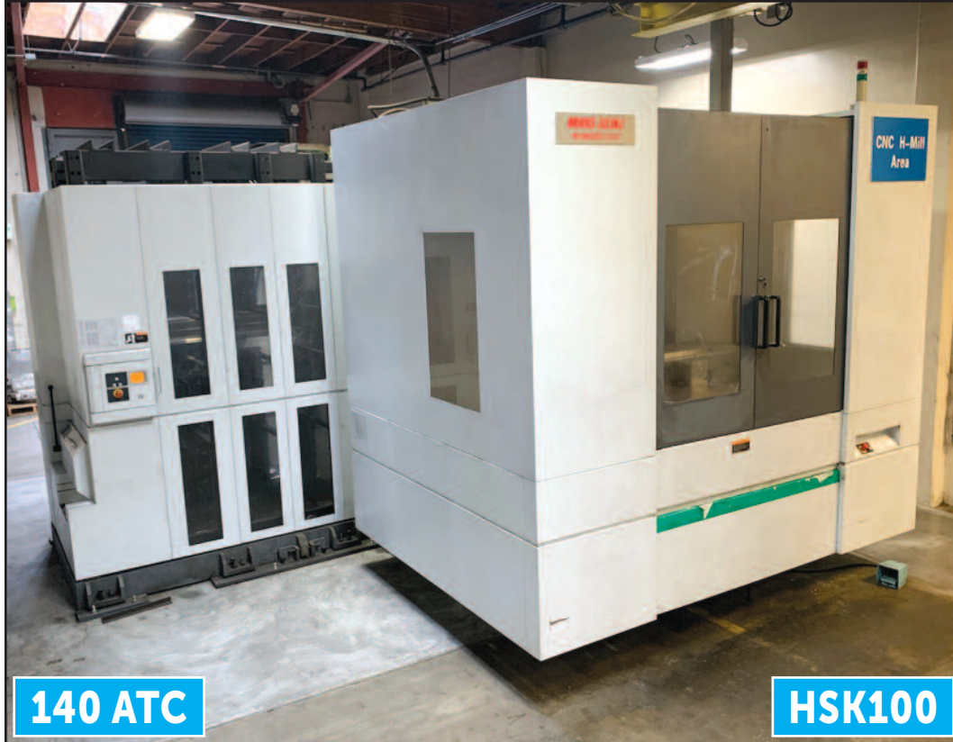
Mori-Seiki NH8000 DCG, 4-Axis, Moric MSX-7011I Control, (2) 31.5" x 31.5" Pallets, 55.1" x 47.2" x 53.1" Travels, .001 Deg. B-Axis, 40 HP, 15K RPM, HSK100 Taper, 140 ATC, Coolant thru Spindle, Chip Conveyor, S/N NH801G10153
