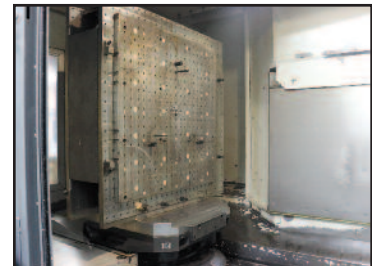
Mori-Seiki NH8000 DCG, 4-Axis, Moric MSX-7011I Control, (2) 31.5" x 31.5" Pallets, 55.1" x 47.2" x 53.1" Travels, .001 Deg. B-Axis, 40 HP, 15K RPM, HSK100 Taper, 140 ATC, Coolant thru Spindle, Chip Conveyor, S/N NH801G10153
