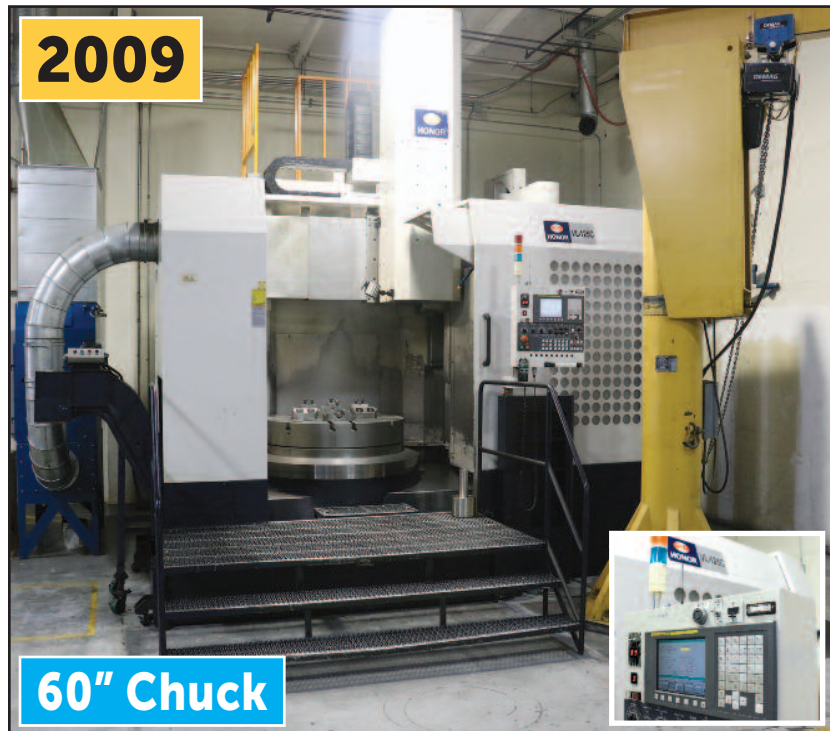
60"/70" Honor-Seiki VL-125C , Fanuc OiTC Control, 12 Position Turret, 6500 Hours
