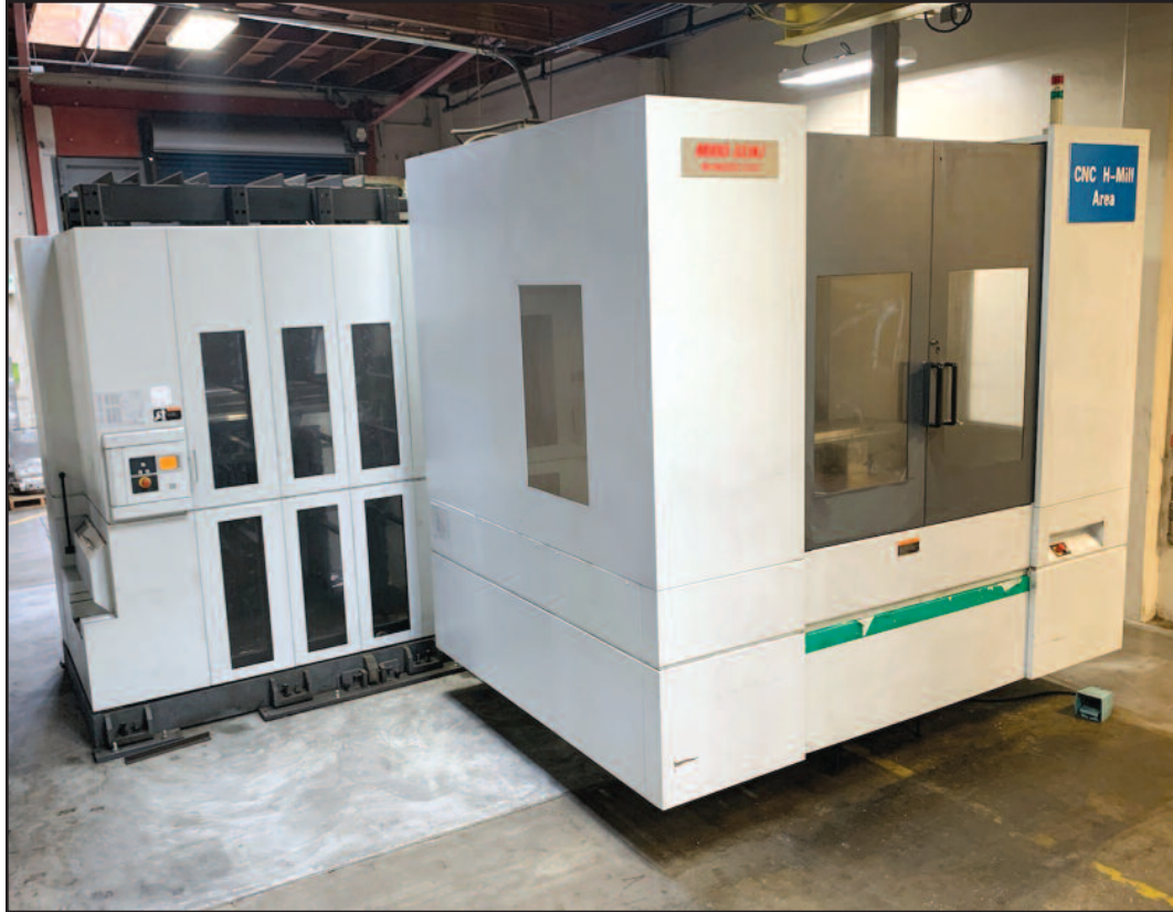
Mori-Seiki NH8000 DCG , 4-Axis, Motic MSX-7011I Control, (2) 31.5" x 31.5" Pallets, 55.1" x 47.2" x 53.1" Travels, .001 Deg. B-Axis, 40 HP, 15K RPM, HSK100 Taper, 140 ATC, Coolant thru Spindle, Chip Conveyor, S/N NH801G10153
