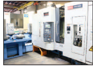
Mori-Seiki NH8000 DCG , 4-Axis, Motic MSX-7011I Control, (2) 31.5" x 31.5" Pallets, 55.1" x 47.2" x 53.1" Travels, .001 Deg. B-Axis, 40 HP, 15K RPM, HSK100 Taper, 140 ATC, Coolant thru Spindle, Chip Conveyor, S/N NH801G10153
