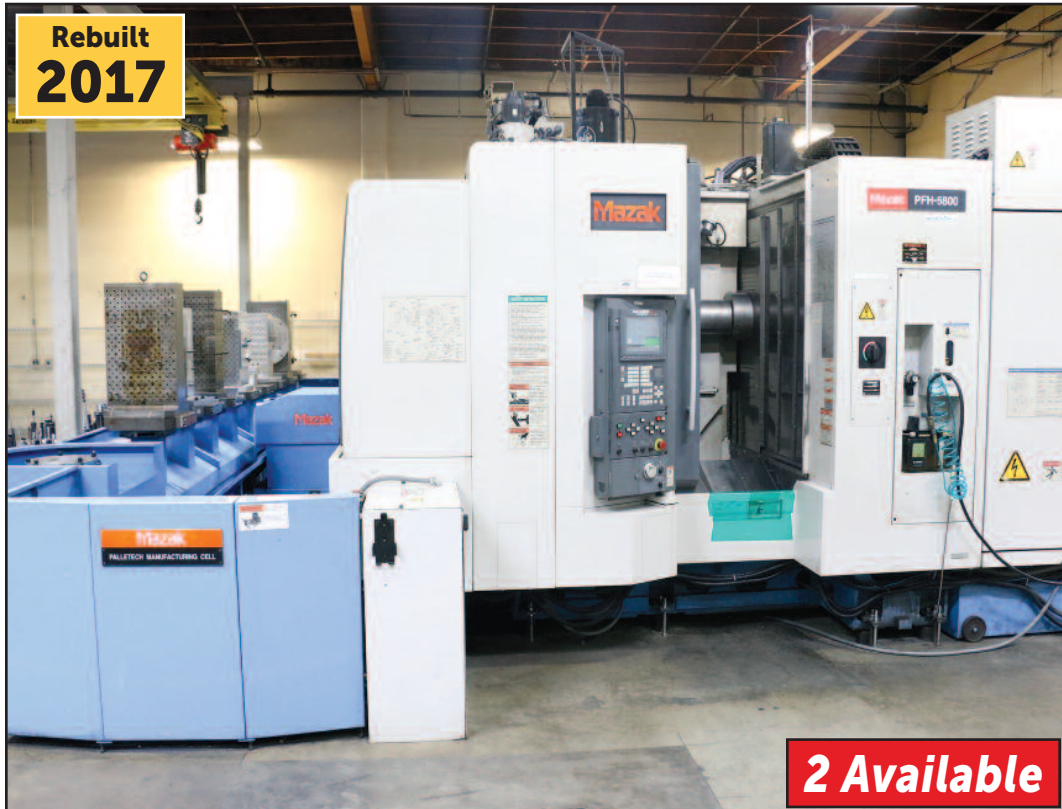
Mazak PFH-5800 , 4-Axis Palletech F.M.S., Fusion 640M Controls, (10) 20" Pallets, 15k RPM, 80 ATC, CTS, Probe, Chip Blaster
