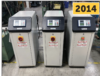
Frigel Microgel Chiller-Temp. Controls
