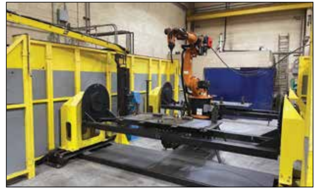
ESAB Swift Arc SL Welding Cells
