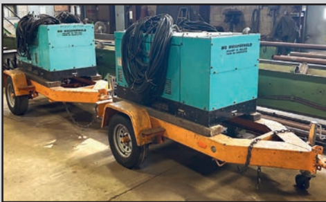
(2) MULTIQUIP DUALWELD 400 DIESEL 14KW WELDING GENERATOR
